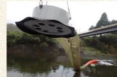
Fig. 1: The Hydro-suction Sediment Removal System mechanism
